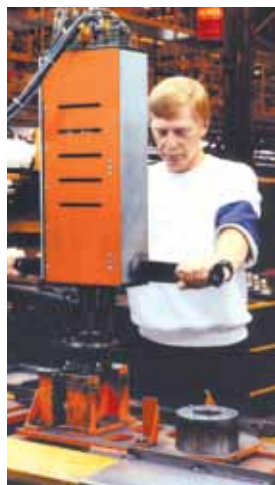
Repair bay operator is using a two spindle fixtured tool to fasten components of a wheel hub assembly.
