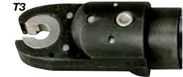
The 48ET tube nut wrench alternates the direction of rotation each time the lever is actuated. When rotating in reverse, the socket will stop at the open position.
